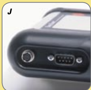
Countersunk connectors, well protected against external damage.
